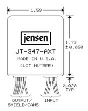
8 INCH #26 AWG (7x34) SILVER PLATED COPPER LEADS WITH TEFLON INSULATION.
