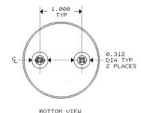
RECOMMENDED MOUNTING IS WITH VR-4 CLAMP (SUPPLIED WITH TRANSFORMER)
